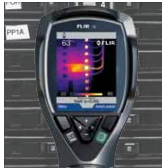
FLIR i3, temperature in 3,600 spots
