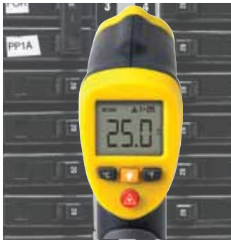
IR thermometer, temperature measurement in one spot
